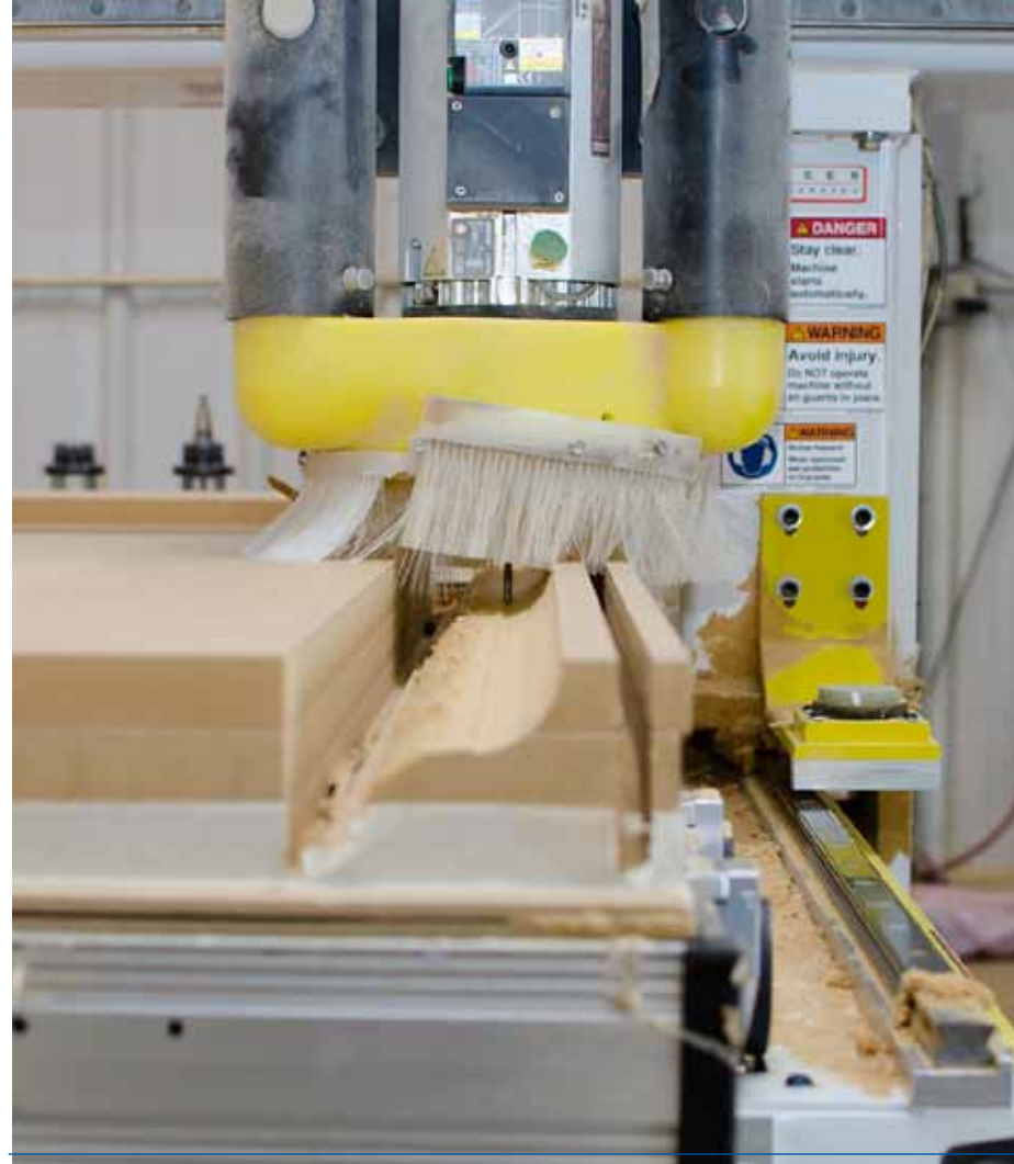
AAS Technology for Creating Customized Molds with Complex Shapes.
